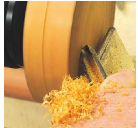
▲ Pic.6 Make the bottom flat or slightly concave. A pull cut with the gouge or a light cut with a scraper is perfect, sliding your hand along the toolrest to guide the tool
